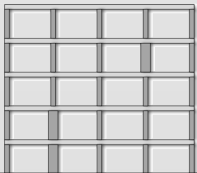
柱斷面勁度變化大
